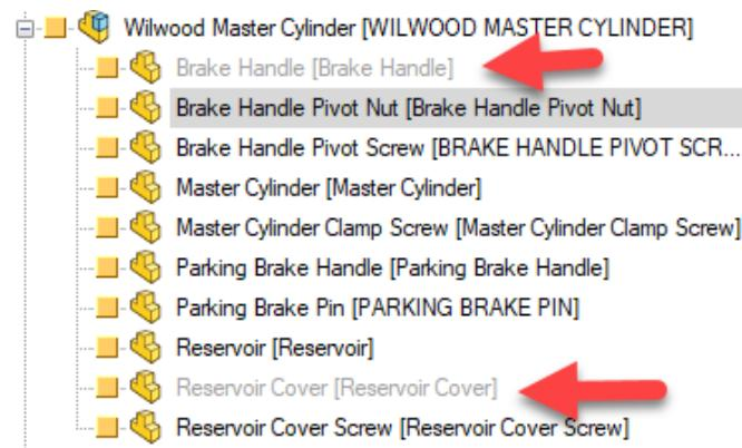
It also has one component (Brake Handle Pivot Nut) with one instance suppressed but not the other:
